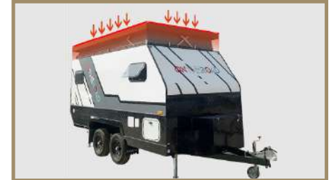
Pop-top roof. higher interior space after roof up.
