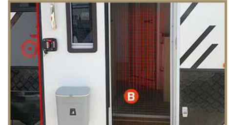
Installed with push-pull screen door.
